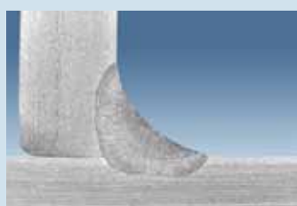
TIG- DC, Argon, v_s = 13 \text{ cm/min}
