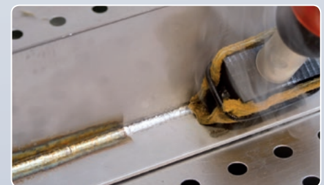
Old method: Welding seam cleaning with tampon
